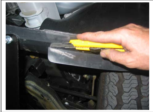
Figure 15 – Cutting flap from inner guard.
