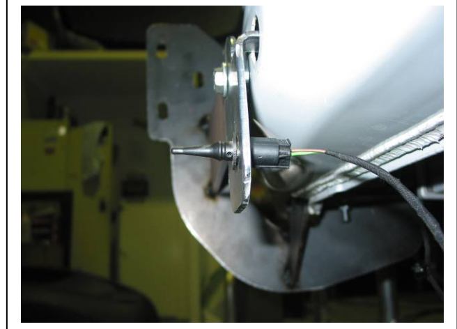
Figure 6: Temperature sensor fitted
