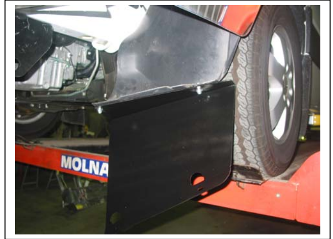
Figure 16 – Under body guard attached to inner guard.
