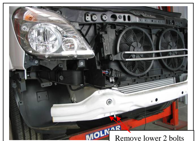
Figure 2: Remove lower two 13mm head bolts
